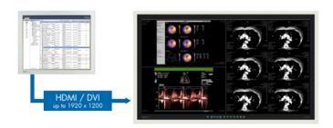
Intel Dual HD graphics chip supports the simultaneous display of two screens with resolutions up to  $1920 \times 1200$  pixels.
